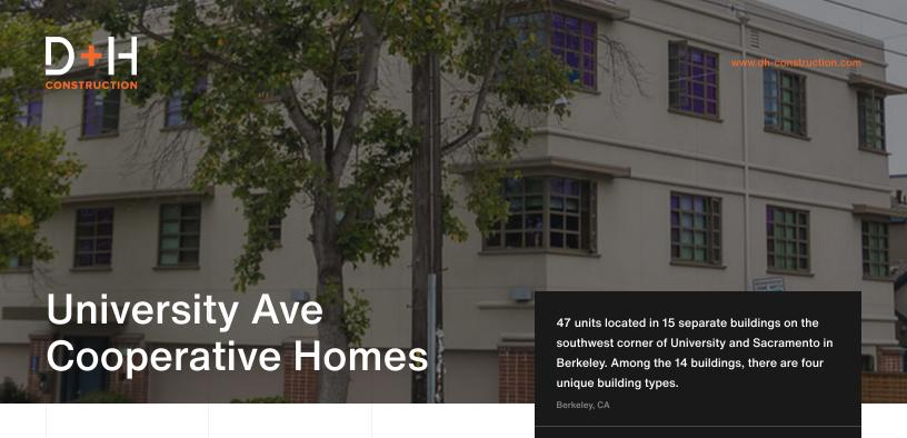
The project included complete interior remodels — kitchens, bathrooms, flooring, and painting — plus installation of new double paned windows, exterior painting, landscaping, elevator upgrades, ADA site work, upgrades to the community room, and adding a photovoltaic system along with new solar thermal system. Since the buildings were occupied, there were five separate phases of the project to accommodate tenant relocation.
